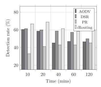
Fig. 2. Malware detection rate in presence of a Nash attacker.
