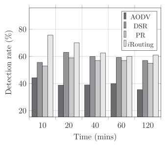
Fig. 3. Malware detection rate in presence of a Uniform attacker.
