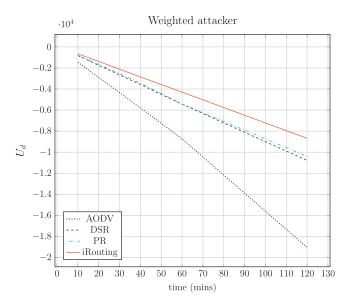
Fig. 7. Utility of the Defender in presence of a Weighted attacker.
