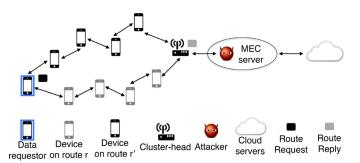
**Fig. 1.** Investigated system model, where a device requests data, that the cluster devices do not possess, from the MEC server. The adversary has successfully launched a MITM attack controlling the communication between cluster-head and MEC server.
