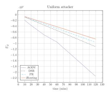
Fig. 6. Utility of the Defender in presence of a Uniform attacker.
