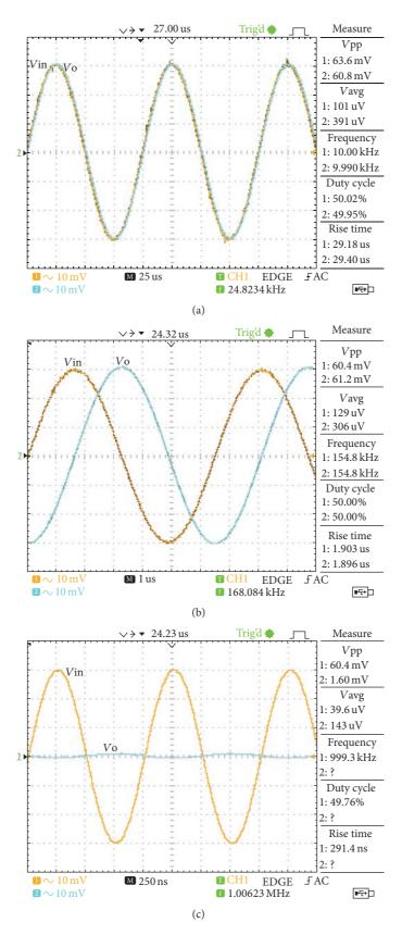
FIGURE 5: The measured input and output waveforms of low-pass filter at (a) 10 kHz, (b) 155 kHz, and (c) 1 MHz.
