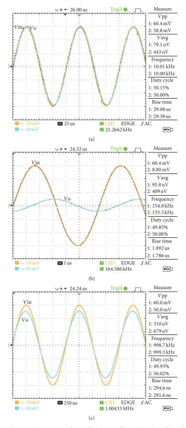
FIGURE 8: The measured input and output waveforms of band-reject filter at (a) 10 kHz, (b) 155 kHz, and (c) 1 MHz.
