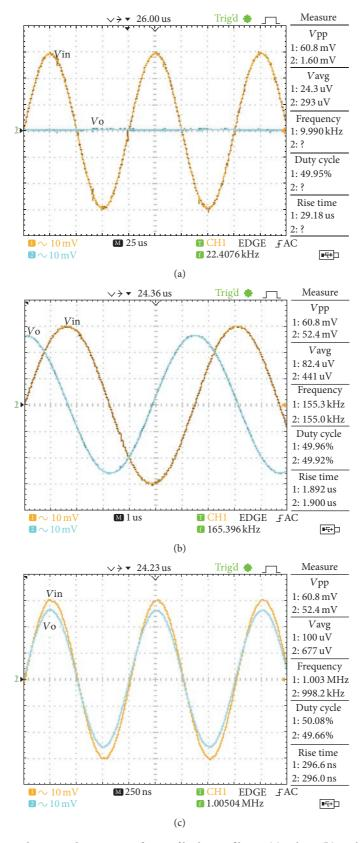
FIGURE 6: The measured input and output waveforms of high-pass filter at (a) 10 kHz, (b) 155 kHz, and (c) 1 MHz.
