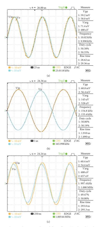
FIGURE 9: The measured input and output waveforms of all-pass filter at (a) 10 kHz, (b) 155 kHz, and (c) 1 MHz.
