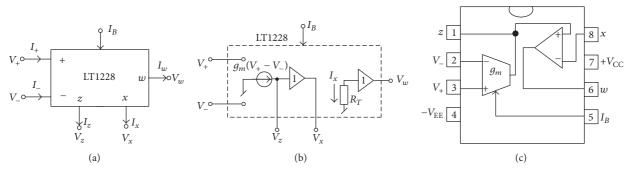
FIGURE 1: LT1228. (a) Electrical symbol of LT1228. (b) Equivalent circuit. (c) Pin configuration.
