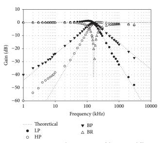
FIGURE 3: Experimental gain response of the proposed filer.
