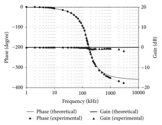
FIGURE 4: Experimental phase and gain response of all-pass function.
