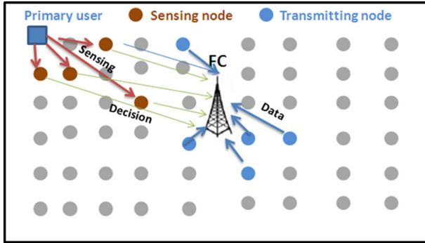
**Fig. 1** Cooperative spectrum sensing and data transmitting configuration
