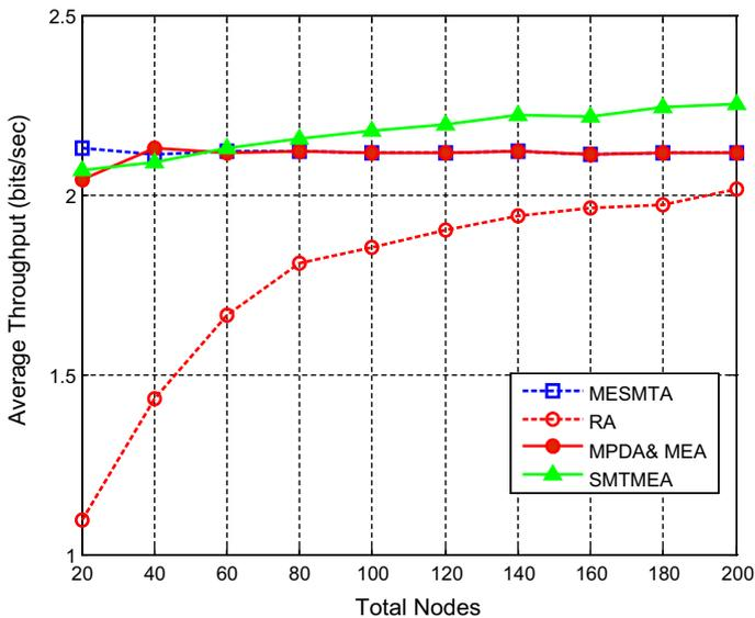
Fig. 7 Average throughput for different number of nodes
