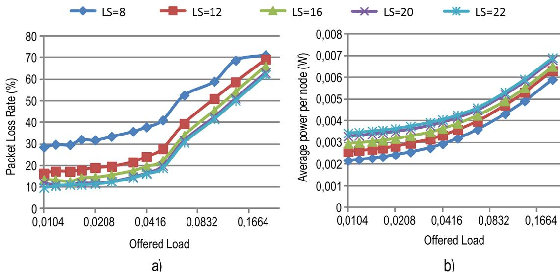
**Fig. 9** Efficiency of the PLOSA protocol according to the number of listening slots. **a** Packet loss rate. **b** Average power per node
