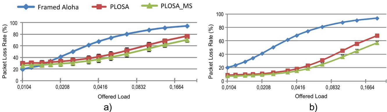
Fig. 4 Packet loss rate under different topologies and densities. a 80-node random topology. b 160-node random topology
