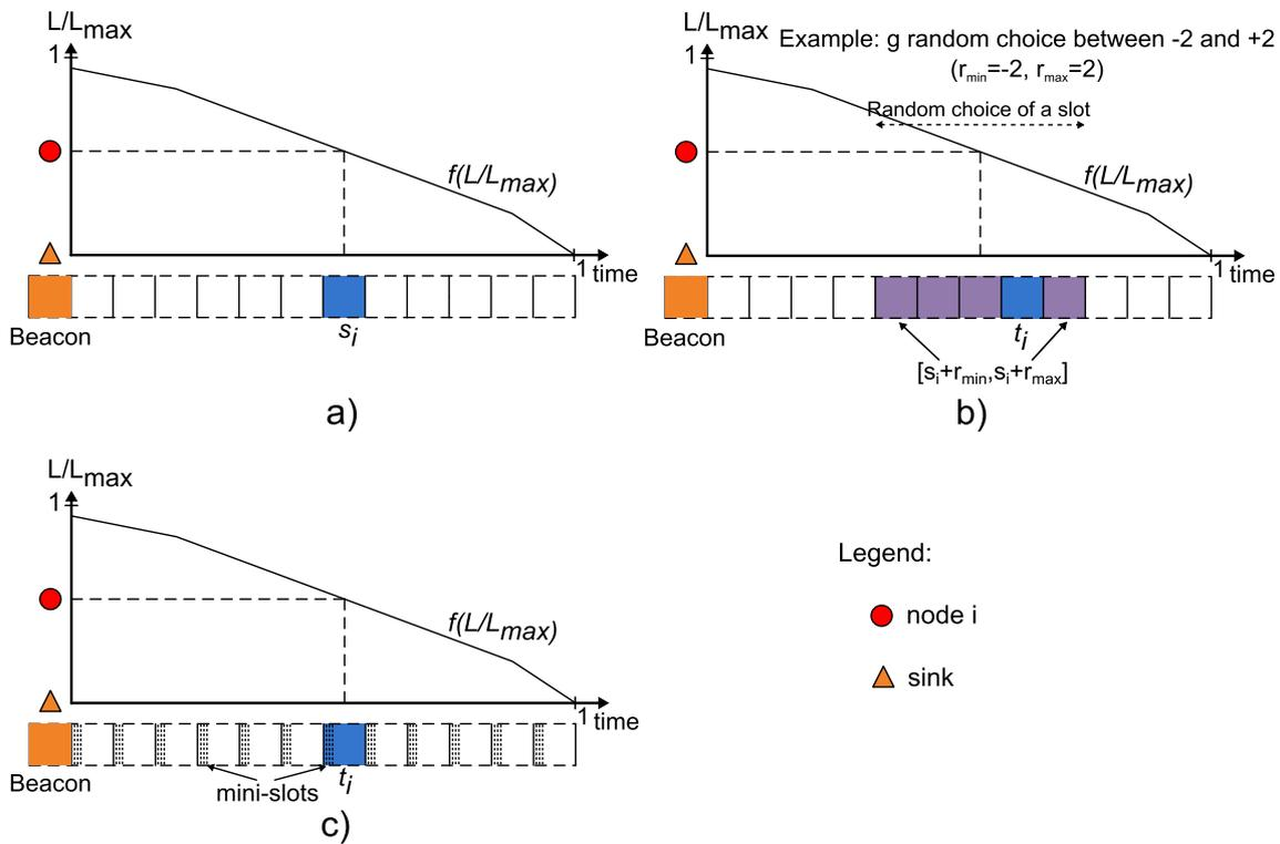
**Fig. 1** Transmission window mechanisms. **a** Main principle. **b** Random slot selection. **c** Mini-slot selection
