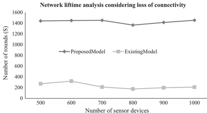
**Fig. 3** Network lifetime analysis considering loss of connectivity for varied sensor devices.
