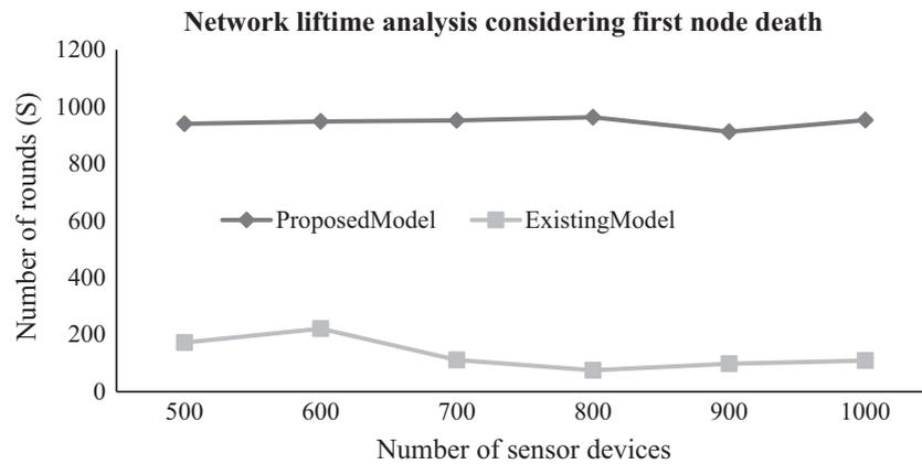
**Fig. 4** Network lifetime analysis considering first node death for varied sensor devices.
