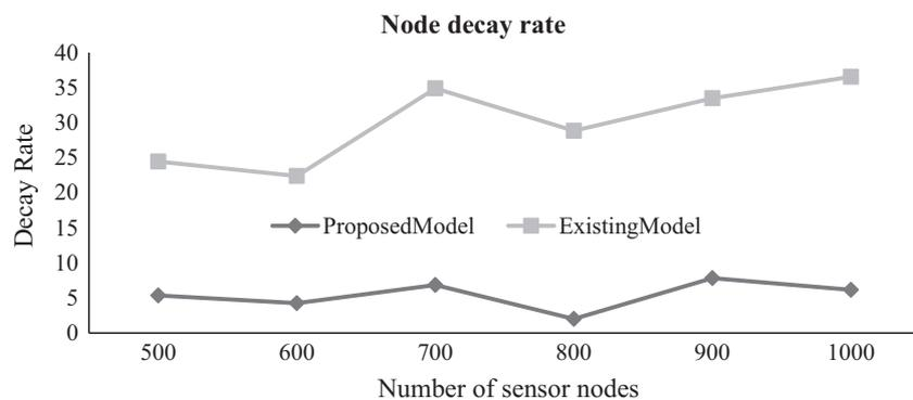
**Fig. 6** Node decay rate considering total node death for varied sensor devices.
