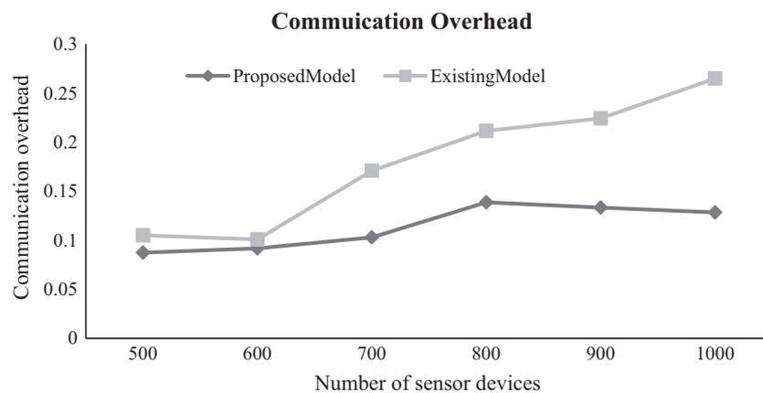
**Fig. 5** Communication overhead considering total node death for varied sensor devices.
